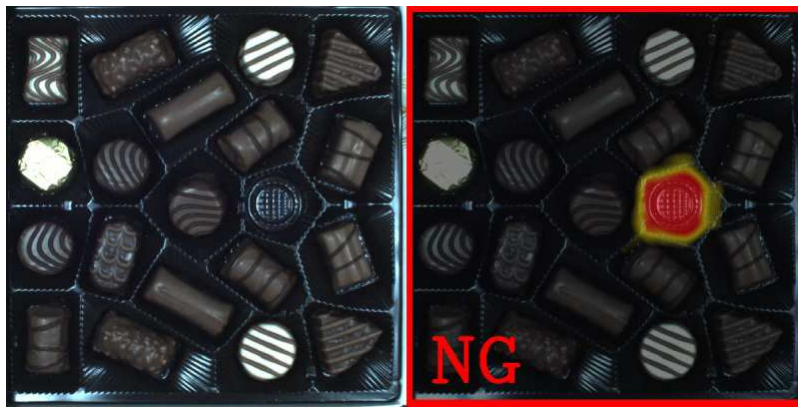
An example of a missing object detection using DL_DetectAnomalies2 tool. Left: The original image with a missing element. Right: The classification result with a heatmap of anomalies.
