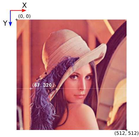
Directions and pixel positions in image coordinates.
