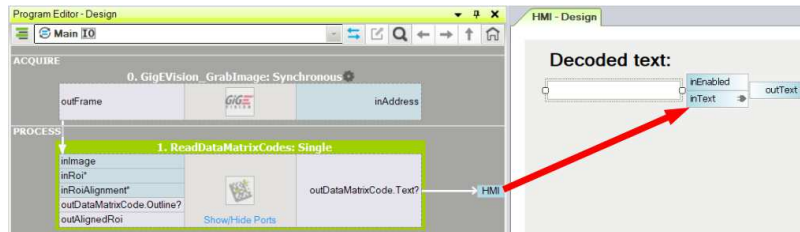
Connection between a filter and a control was established.
