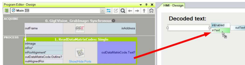
Connecting a filter with a control.
