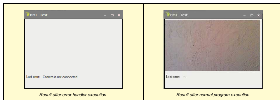
Sample program with error handler. Macrofilter GrabImage has error handler IO_ERROR (right) with error message.
