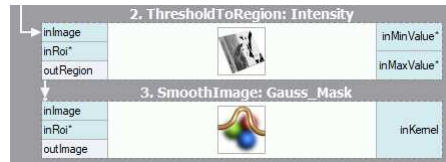
A typical example of automatic conversion: a region being used as an image.
