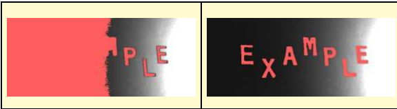
Results of ThresholdToRegion and ThresholdToRegion_Dynamic on images with uneven light.
